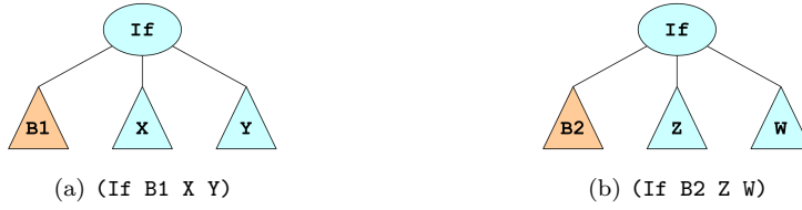
Fig. 9 Distance calculation: Example 3. Two If expressions, wherein distance calculation has to take several edit scripts into account.
