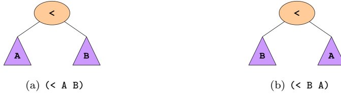
Fig. 8 Two less-than expressions, with identical children in reverse order. (a) is not equivalent to the negation of (b) since both return false in the case of A and B returning the same value.
