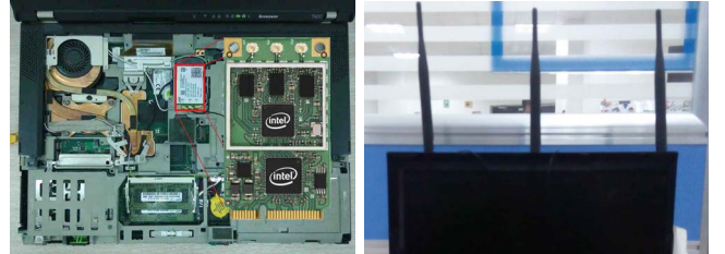
Figure 9: Thinkpad T400 with Intel 5300 NIC, which has three antennae and reports CSI of 30 subcarriers on each antenna.
