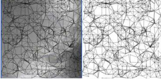
Fig. 2. VG of 450 RSs (10m antenna heights and 10 km transmission range). On the left: VG displayed over  $100 \times 100 \text{ km}^2$  DEM (the lighter the higher). On the right: the same VG displayed with the DEM hidden.)
