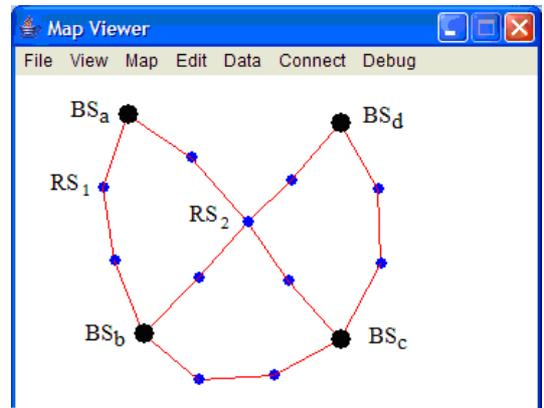
Fig. 1. Four BSs (big circles) and 11 RS (small circles) example: The optimal solution is 5 (using the middle RS), while any solution based on shortest path like method is 6 (using the outer RSs).
