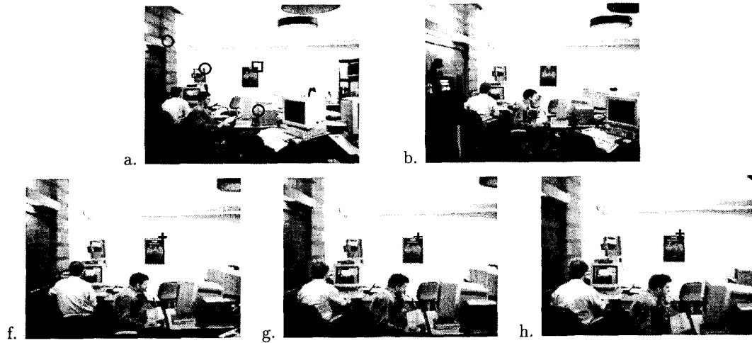
Figure 2: The top row shows two training images taken about one meter apart with the robot looking in the same direction. The remaining images were taken at equal intervals as the robot moved forward approximately ten feet from its position in Figure b. During training the image coordinates of all four features marked in Figure 2.a were known initially, then tracked to their positions in Figure 2.b. The crosses in the subsequent three images indicate the robot's predictions of the feature location.
