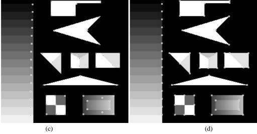
Figure 2: Corner maps of the synthetic image obtained by: (a) New Algorithm; (b) Wang and Brady Corner Detector; (c) Plessey Corner Detector; (d) SUSAN Corner Detector
