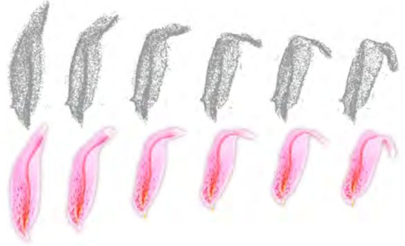
Figure 8: Tracking and fitting a single petal. The captured point clouds at different time steps (top) are tracked and fit by a petal template model (bottom) using data fitting and shape preservation.
