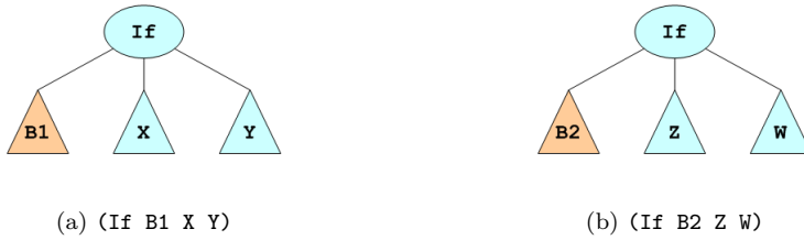
Fig. 9 Distance calculation: Example 3. Two If expressions, wherein distance calculation has to take several edit scripts into account.
