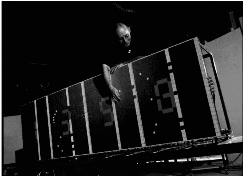
Figure 1: The BioWall, an interactive reconfigurable computing tissue of 80 \times 25 = 2000 cells (Photograph by A. Herzog).
