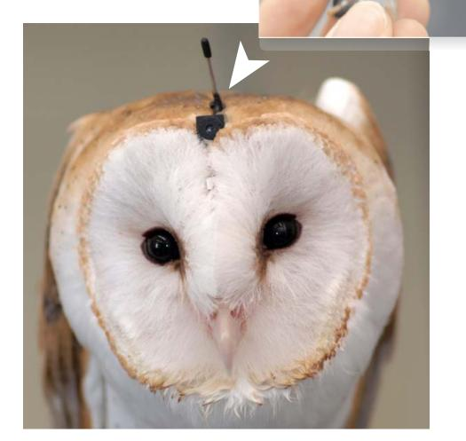
The **OwlCam** is a tiny and lightweight wireless video camera mounted onto the head of a barn owl. Images from the OwlCam align with the animal's gaze because barn owls lack eye movements
