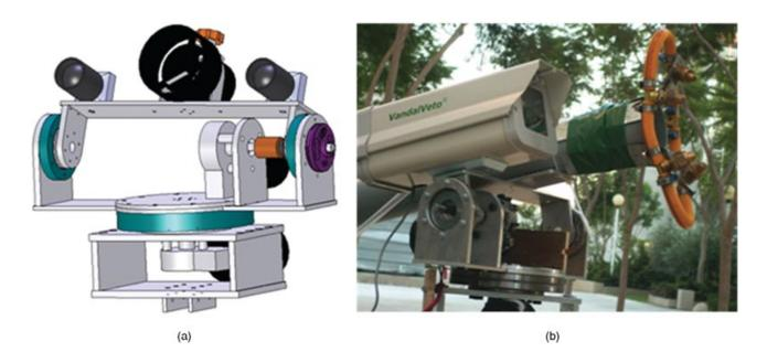
Figure 4. (a) The design model of the spraying head. (b) The actual head used in our experiments.
