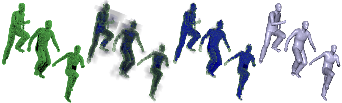
Figure 1: Reconstruction of a space-time surface. Left: A sequence of point clouds of a running man containing holes due to self occlusions. Middle: Renderings of two iterations of our flow solver. Cells confidently identified as being inside the surface are colored dark blue. As the solver progresses, mass accumulates inside the surface. Right: The result of an implicit function reconstruction from the flow solution.
