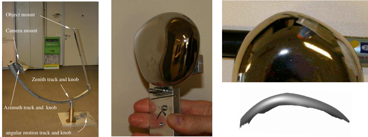
Figure 6. Results with captured data. Left: Acquisition system that enables camera/object rotation about arbitrary axes. Middle: Object under study. Right: Shape recovered from two specular flows, shown with a comparable view of the object.
