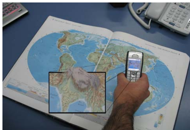
Fig. 1 In-Place Augmented Reality demonstrated using a physical map from an atlas book. Note the elevation of Tibet. The terrain model is extracted according to the colors of the map and augmented back onto the book with no requirement for a content library. The mobile device illustrates a possible platform of usage
