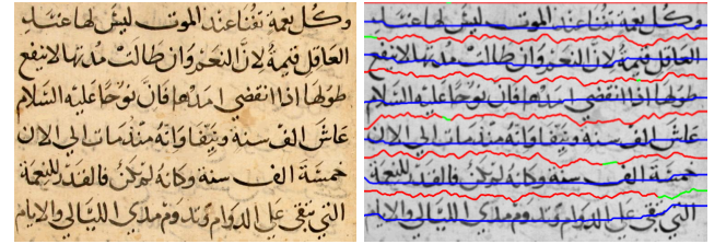
Figure 7: The last word on the second line(right-to-left), descender besieges the propagating seam and force it to pass through.
