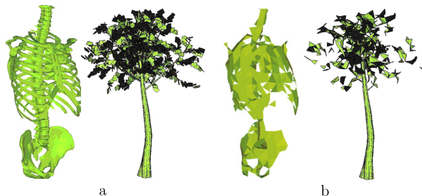
Fig. 1. The effect of the pair-collapse operator on a topologically complex model and a highly clustered non-manifold model: (a) Original models, (b) pair-collapse simplified models. Note the increased number of disconnected components and shrunk appearance.
